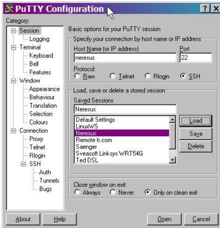
Figure 2: Loading a previously saved configuration, these settings will connection to a host named 'neresus' on port 22 using ssh.
