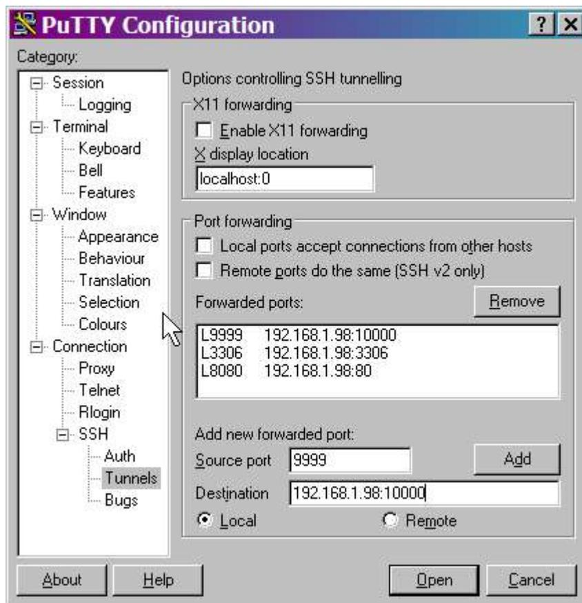
Figure 1: Sample PuTTY configuration with three ports forwarded to local machine. Textboxes are filled in to show how the first entry was created.
